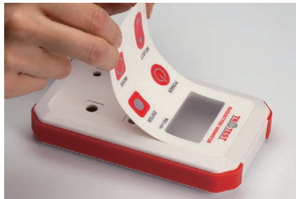
8. Sticking overlay sheet onto enclosure
