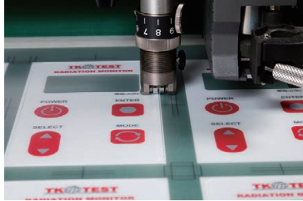
5. Cutting the sheet to size
